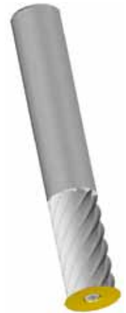
Ensemble fraise HSS et couteau CW Combination of HSS shredder and WC cutter
